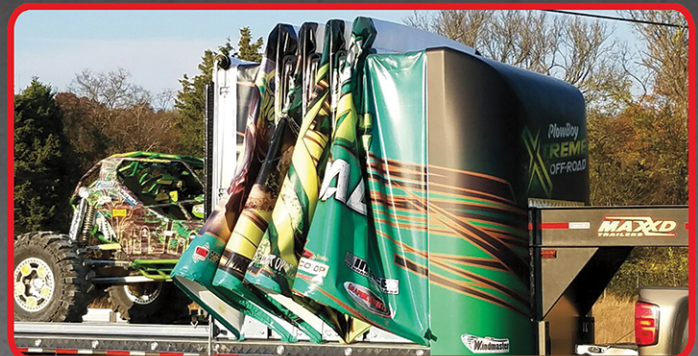
Fiberglass Windmaster Aerodynamic Bulkhead Finishes Off the Front Of Trailer
