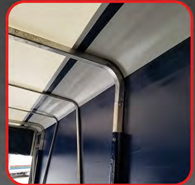
Alum. Roll Formed Bent Tube Frame Construction w/ tight interior Radius
