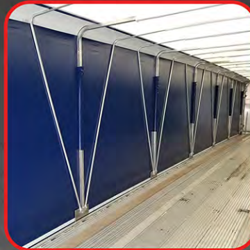
One Pcs. Tarp Construction with Full Length White Skylight and Double Uplift Bows
