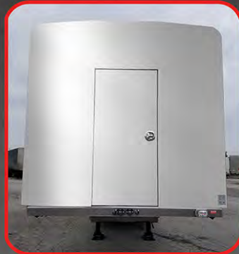
Chamfered Bulkhead with 6ft Man Door sits flush on deck
